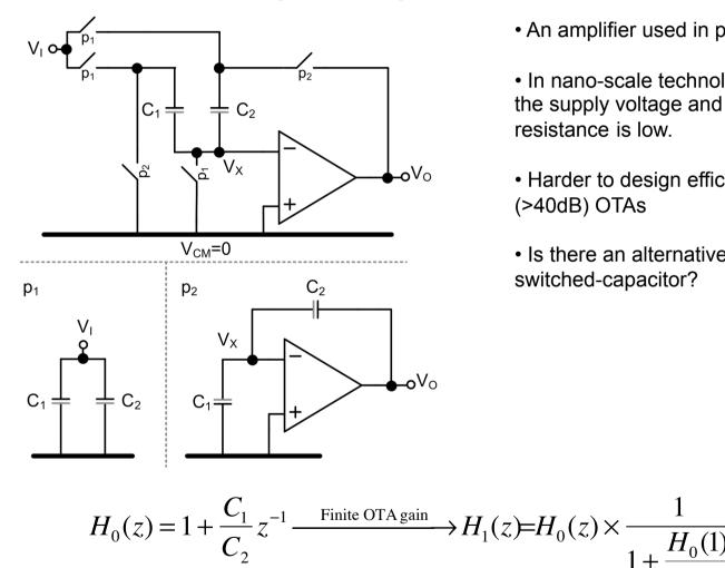
An amplifier used in pipelined ADCs
